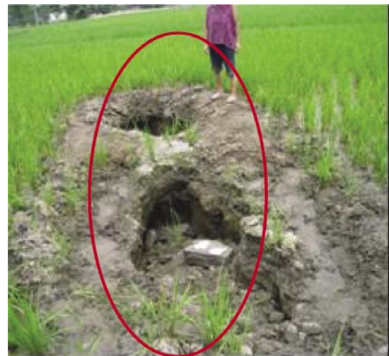
Fig. 7 Large pits of about 3 to 5m in diameter (left) and ground failure (right) were created by water/sand ejection in Xiangliu Village (Photo by WM Wang)
