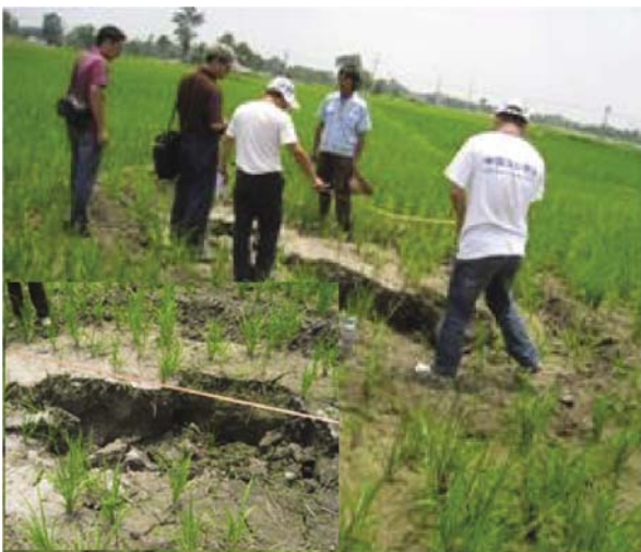
Fig. 7 Large pits of about 3 to 5m in diameter (left) and ground failure (right) were created by water/sand ejection in Xiangliu Village (Photo by WM Wang)
