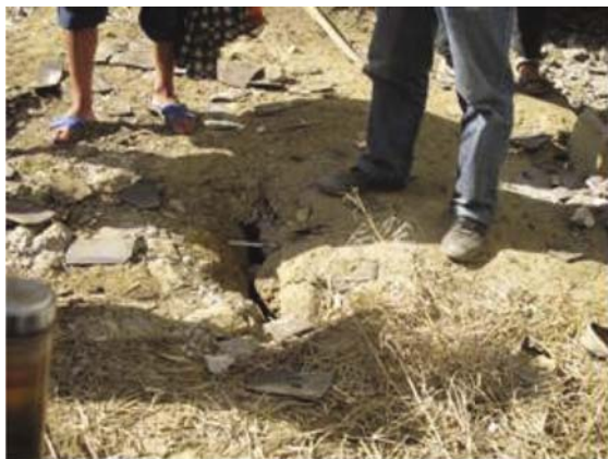
Fig. 15 Liquefaction reoccurrence following the aftershock (left) and subsidence of the house adjacent (right) (Photo by WM Wang)
