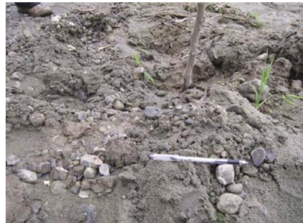
Fig. 13 Gravelly sand of 3 cm to 15 cm in diameter ejected to the ground (Photo by SY Li and ZZ Cao)
