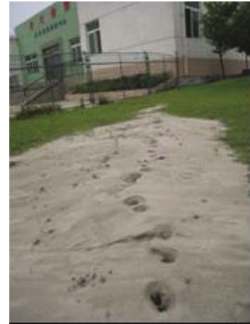
Fig. 5 Large sand boil (left) and aligned sand boils along the crack in the ground (right) in Mianyang area (Photo by ZZ Cao)
