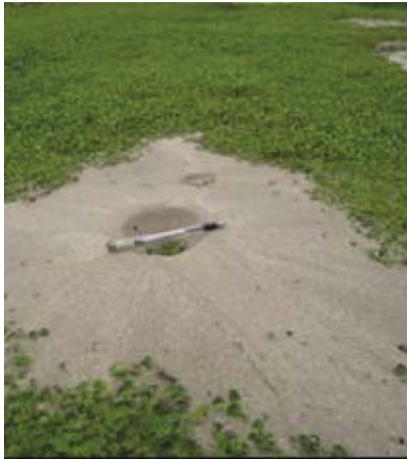
Fig. 5 Large sand boil (left) and aligned sand boils along the crack in the ground (right) in Mianyang area (Photo by ZZ Cao)
