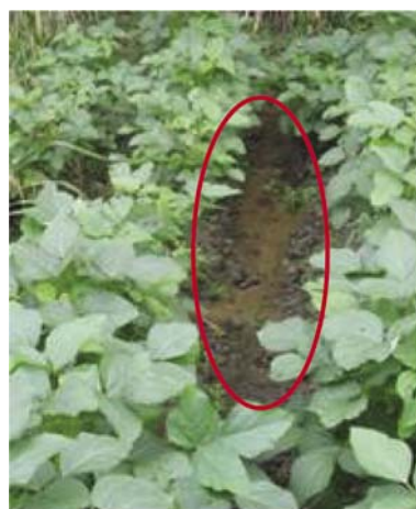
Fig. 4 Yellow ejected sand and water in Xinlian Village of Leshan City, where water spouting lasted more than 3 months (Photo by LW Chen)
