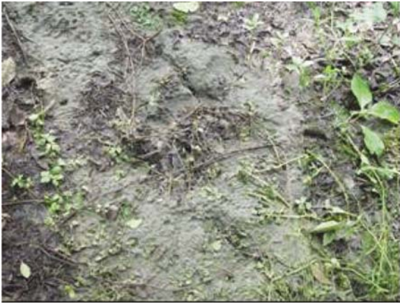
Fig. 11 Grey and yellow fine sand ejected to the ground following liquefaction behaviors (Photo by JS Bo and ZZ Cao)
