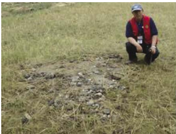
Fig. 13 Gravelly sand of 3 cm to 15 cm in diameter ejected to the ground (Photo by SY Li and ZZ Cao)
